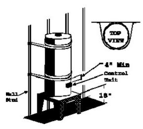
Drill pilot holes on the centerline of the stud (both sides of the heater), Insert screws through punched holes in the strap.
